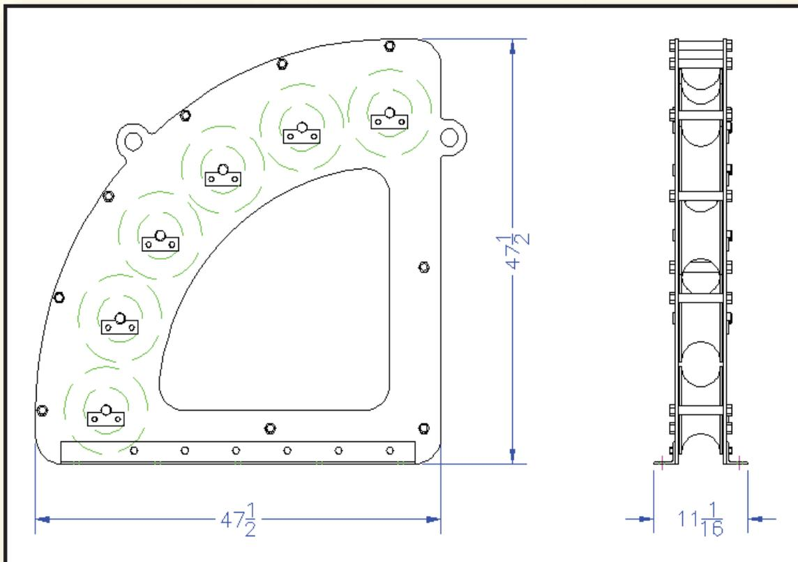
*Typical configuration for 36" bend radius with 3 1/2" cable diameter. Due to our policy of continuing development, all specifications are subject to change without notice. Users of these products are responsible for ensuring their suitability for the application in which they are being used.*
