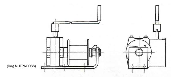
\* 'P' designates winch may be used with power, reducing rated capacity by 50%. Use intermittent power only. See 'OPERATION' for duty cycle. Motor is customer-provided.
